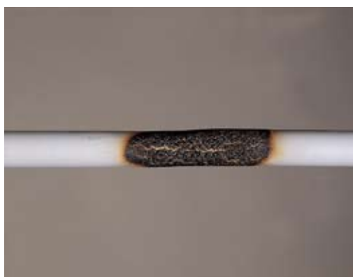
CPVC - After torch is removed
