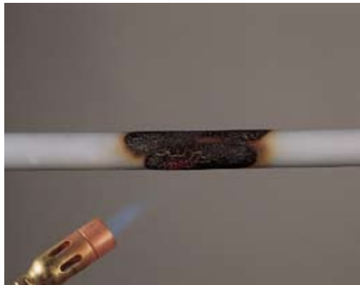
CPVC - initially when torch is applied
